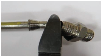
Figure 32: Wire from the LT102B being cut at the pin receiver.
