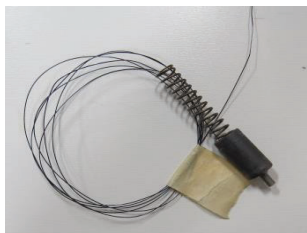
Figure 34: Coil the trigger, spring, and wire to be packaged for return to McNeilus Warranty.
