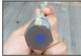
Figure 41: Blue dot indicates the trigger line has been inspected and is suitable for use.
