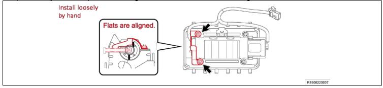
Push the inflator and plate to towards the position determining plate to eliminate any gap.
