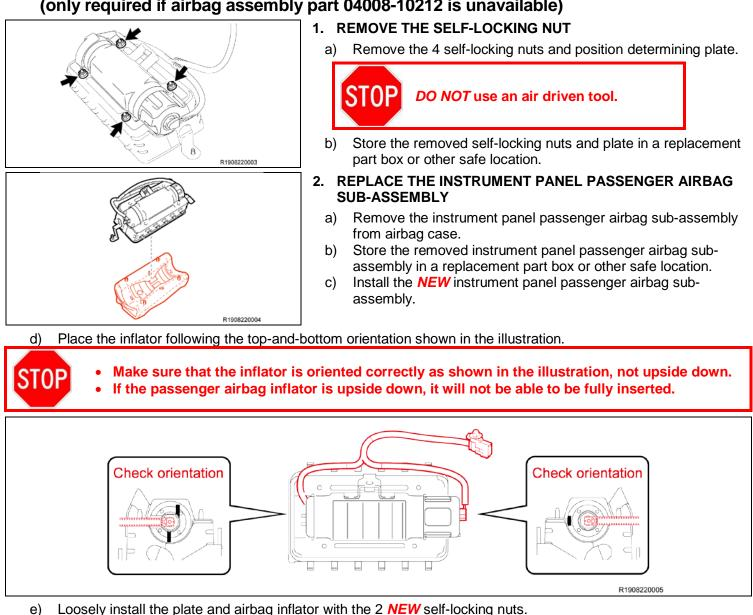
Loosely install the plate and airbag inflator with the 2 NEW self-locking nuts.
