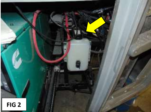
FIG 1: Open the generator compartment using the switch (arrow) inside the driver side front electrical compartment. FIG 2: Bolt is located on the right side of the generator behind the washer fluid bottle (arrow).
