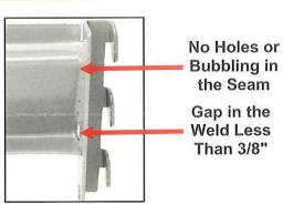
A good beam will have a proper weld along the diagonal following the seam. There will be no visible gaps in the diagonal weld, and there may be one minimal gap in the bend that will measure 3/8" or less.
