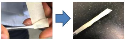
4. Place the clean micro fiber between the pole guide and the front seat-back.
