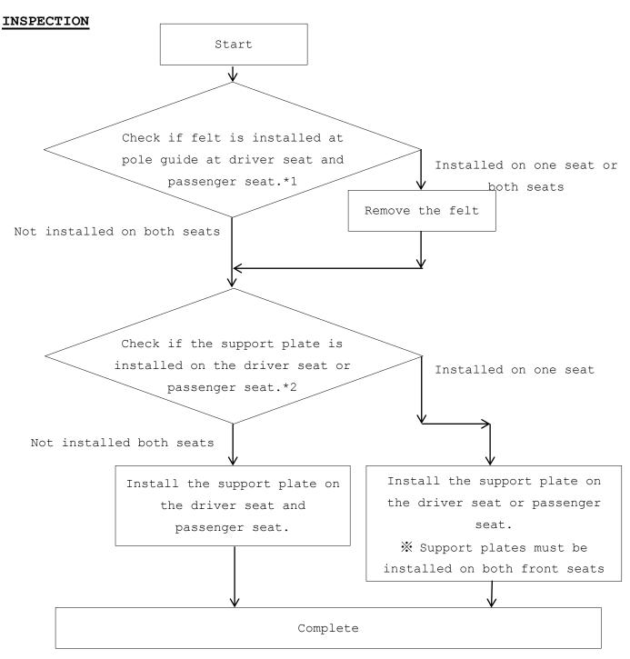
\*1 Some vehicles (about 700 VINs) had felt installed which was a temporary measure to avoid pushing the release knob. \*2 Some vehicles (about 360 VIN) were installed with the support plate on the driver seat or passenger seat.
