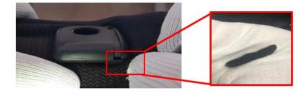
3. Use a regular flat screwdriver and apply masking tape to prevent damage the trim and pole guide.
