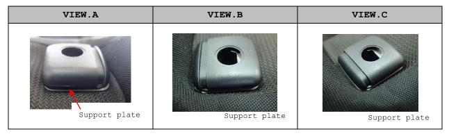
Install the support plate on the driver seat and/or passenger seat.
