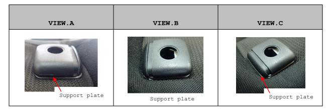
6. Install the support plate on the other seat (passenger seat).
