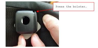
5. While pressing the bolster, fit the ribs of the pole guide with the support plate.
