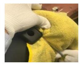
6. Take the felt with a finger and remove the micro fiber. Be sure to remove all of the felt.
