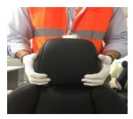
9. Push the head rest down direction and verify that the head rest does not unlock each notch.
