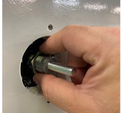
Place the cup over the latch mechanism with the two rivet holes lining up in the vertical position. Predrill the fiberglass through the rivet holes in the cup. Be careful not to drill too deep and contact the exterior skin. A hole just through the fiberglass is sufficient. Rivet the cup in place. From the interior side, place one large washer and one large nut on the latch mechanism and tighten to the cup.
