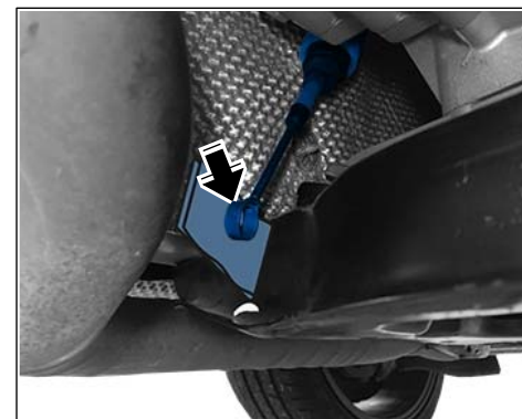
Cleaning bore on pendulum joint
