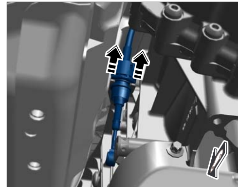
Pulling out selector lever cable
