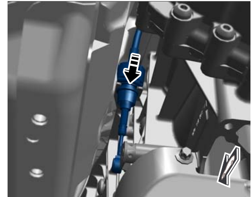
Pushing in selector lever cable
