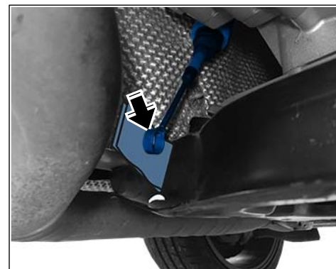
Cleaning bore on pendulum joint
