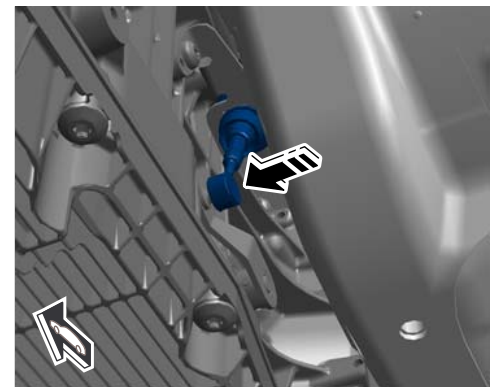
Pressing in selector lever cable
