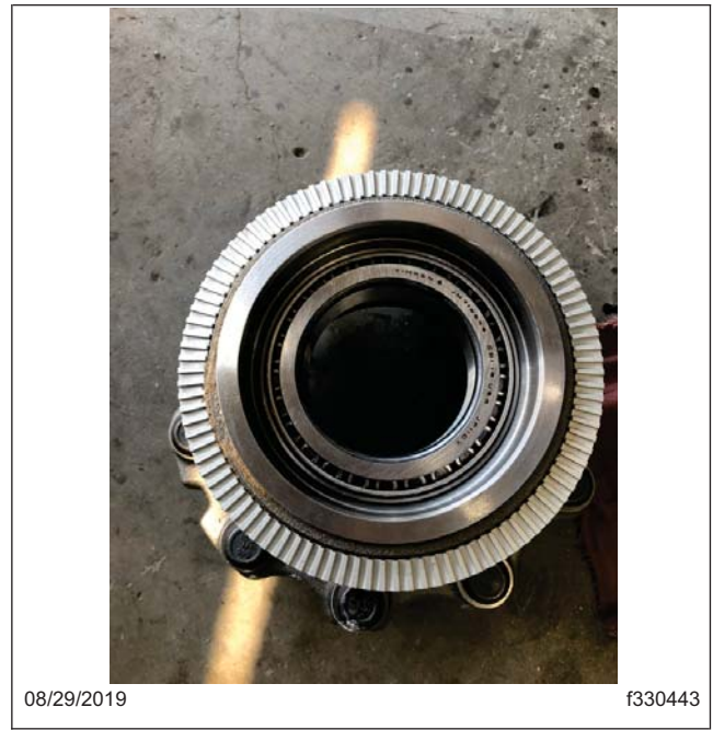
Fig. 24, Lubricated New Inner Wheel Bearing
