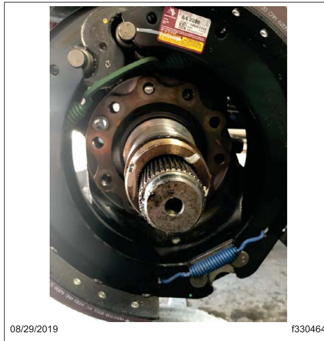
Fig. 19, Removed Mounting Flange Bolt
