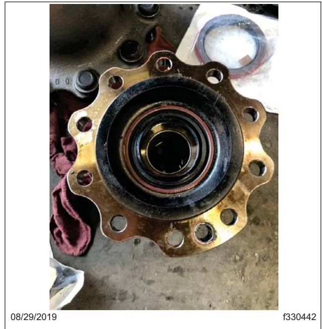
Fig. 22, Installed Spindle Seal
