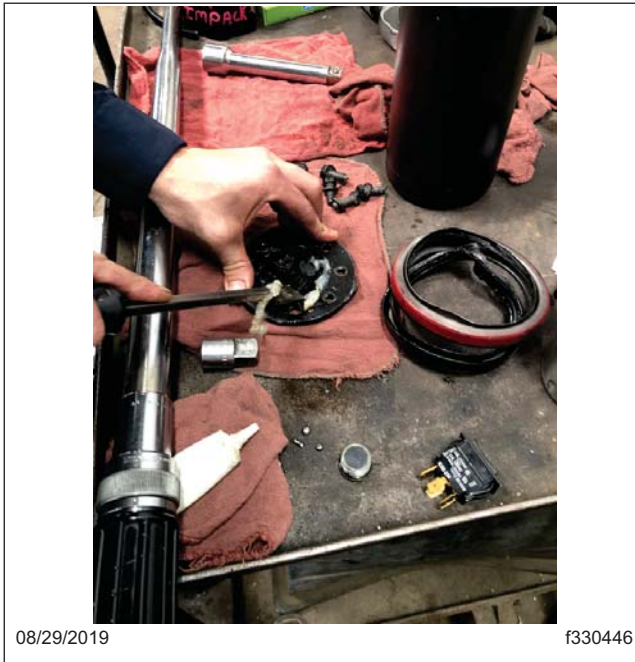
Fig. 27, Cleaning the Hub Cover
