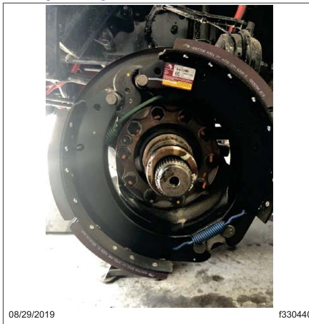
Fig. 14, Removed Hub and Inner Bearing
