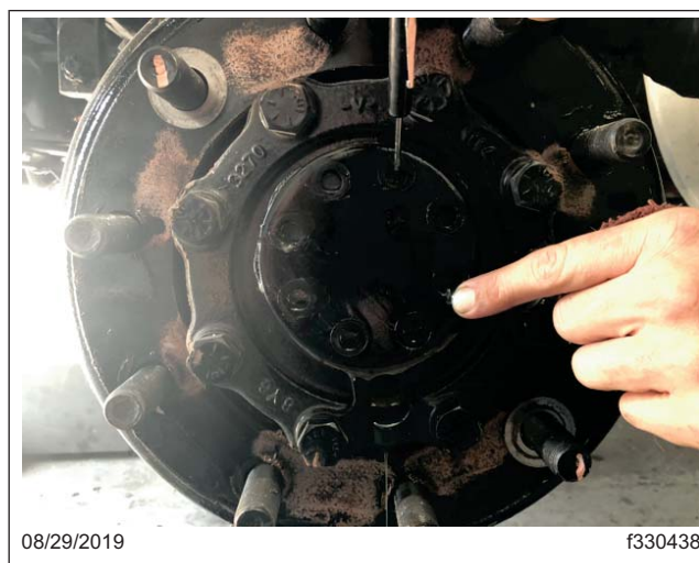
Fig. 2, Removed Hub Cover Bolts
