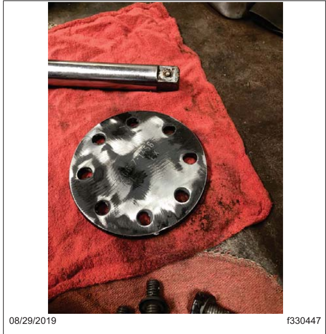
Fig. 28, Cleaned Hub Cover
