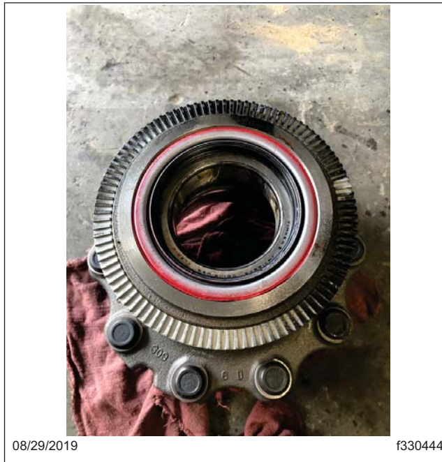
Fig. 25, Installed Hub Seal
