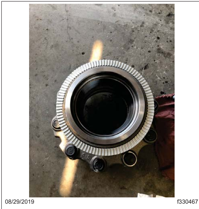
Fig. 23, Lubricating the New Inner Wheel Bearing
