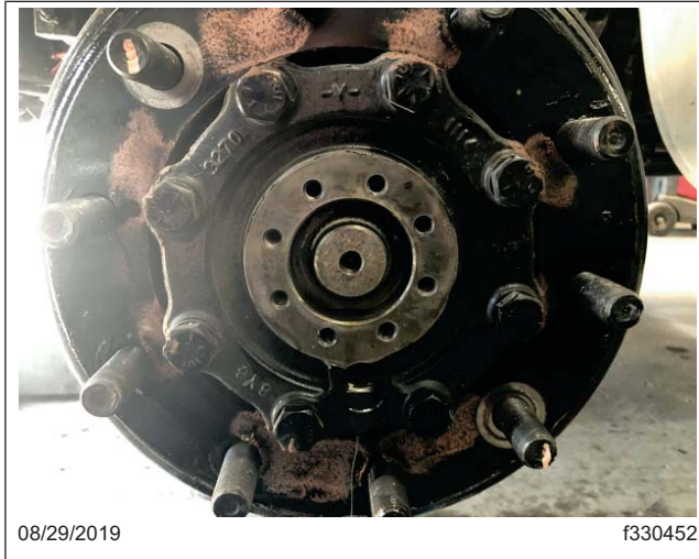
Fig. 6, Flange Bolts Connecting the Drive Flange to the Wheel Hub
