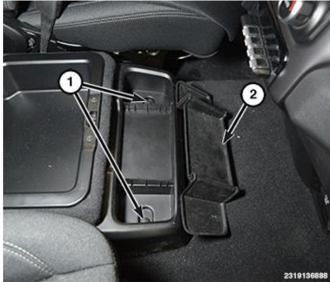
Figure 7 – Storage Bin Liner and Fasteners
