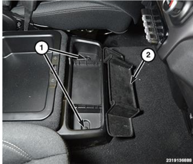
Figure 7 – Storage Bin Liner and Fasteners
