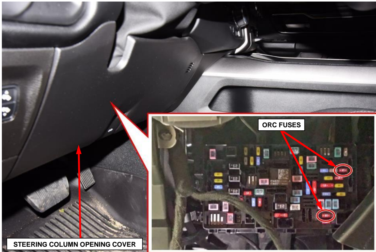
Figure 16 – ORC Fuses F28 and F65
