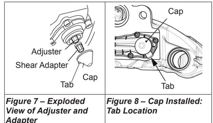
2. For illustration purposes, the exploded view (*Figure 7*) shows the adjuster and shear adapter separated. When using the adjuster mechanism, always have the shear adapter installed on the adjuster.
