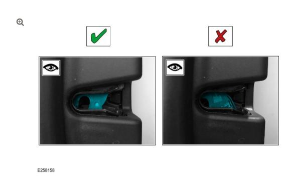
Use a quick and smooth motion to grasp and pull the exterior door handle, hold the handle in the open/extended position, and observe the position of the door latch lever.
