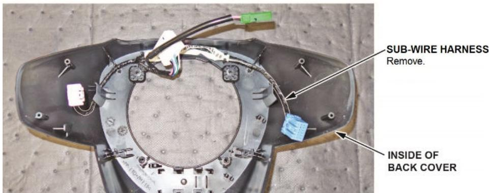
20. Check the sub-wire harness part label to be sure you have the correct part for the trim level you are repairing. **Make sure it is the same part number as the one you are replacing.**
