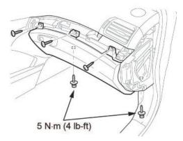
4. Pull the glove box out to detach the clips.
