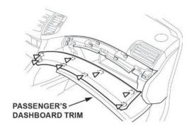
3. Close the glove box, and remove the bolts and screws.
