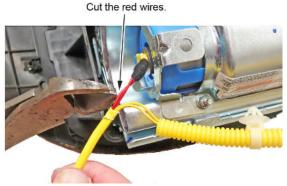
3.2. Strip away about 1 inch of the red wire insulation, then twist the wires together.
