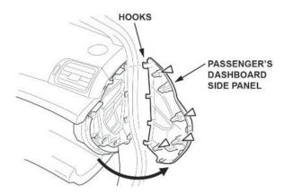
2. Open the glove box, and remove the passenger's dashboard trim.
