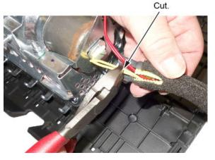
3.5. Strip away about 1 inch of the yellow wire insulation, then twist the wires together.
