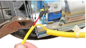
3.2. Strip away about 1 inch of the red wire insulation, then twist the wires together.
