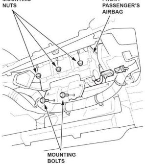
9. Release the pins and remove the front passenger's airbag.
