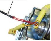
3.3. Tape the twisted ends with electrical tape.
