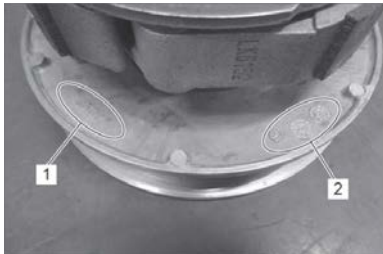
Original production driven face set NO blue paint between the two casting impressions (1 and 2)
