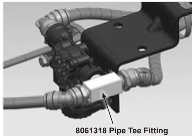
Figure 4, Revised Installation at ABS Modulator
