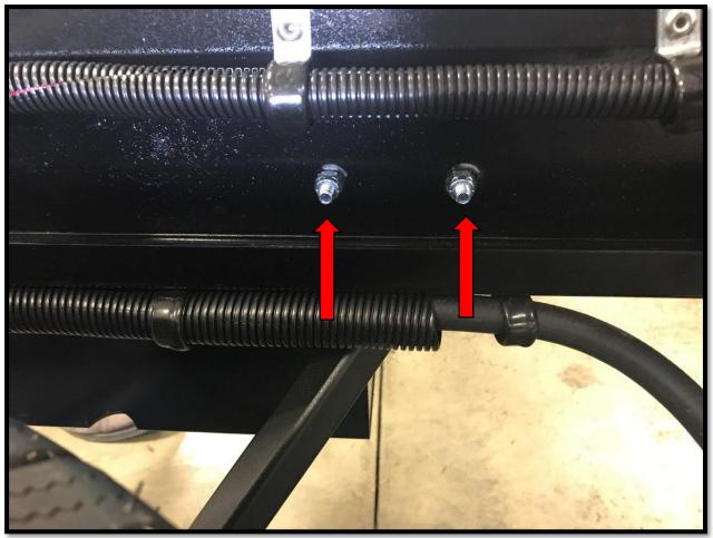
**<u>Step 4:</u>** Using the nuts and bolts removed, attach the new spare tire bracket (Part # **450414-02**).
