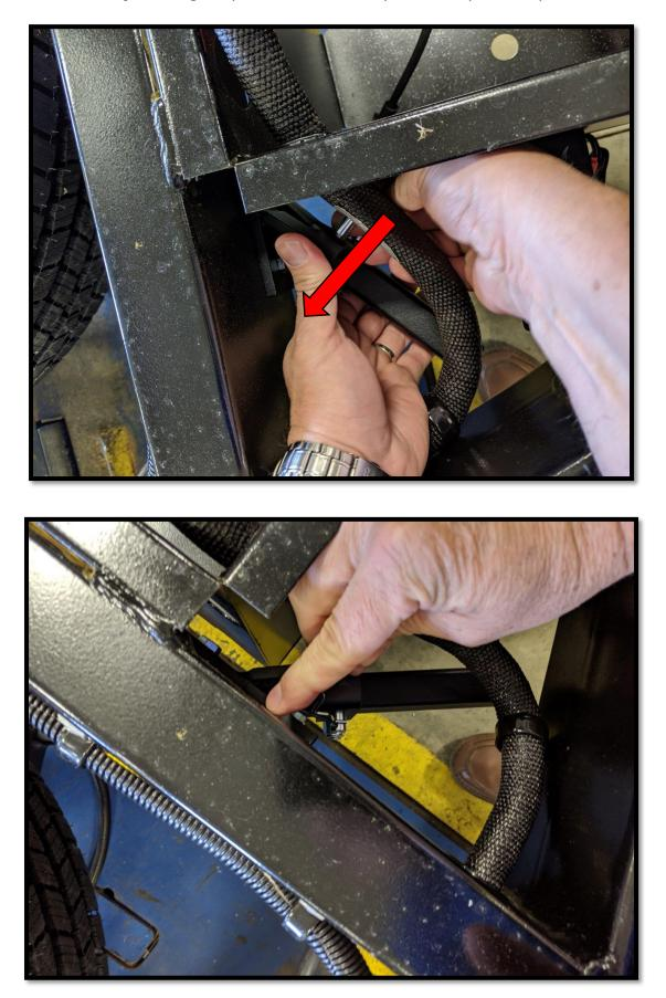
**<u>Step 5:</u>** Using the pivot arm, raise the spare tire, replace the pins.
