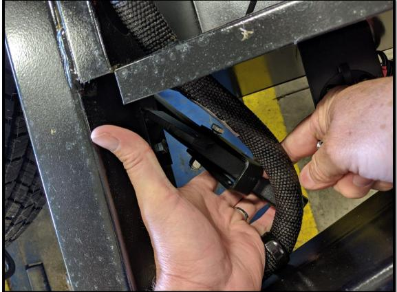
**Step 3:** After you have the spare tire lowered, locate the 5/16" nuts on the back side of the spare tire bracket. Remove the nuts and the bolts and remove the existing spare tire bracket.
