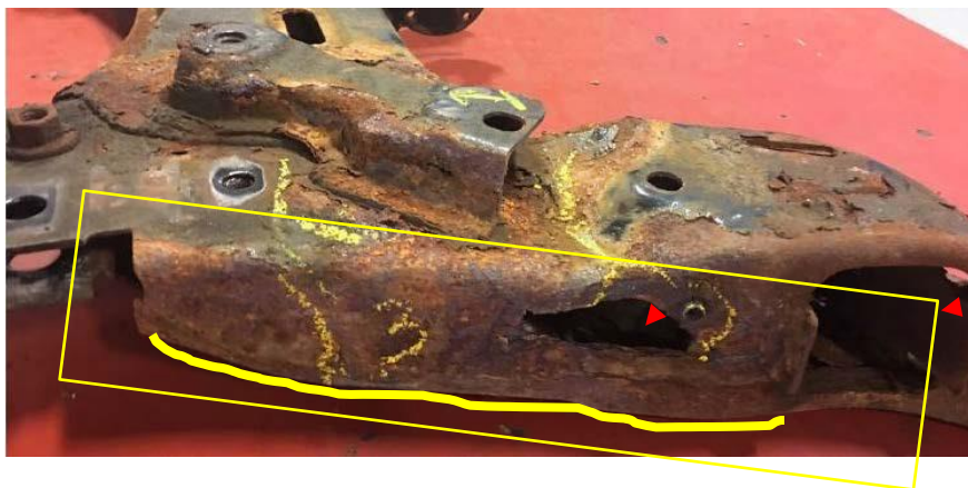
Top Side View: Damaged Cross member
