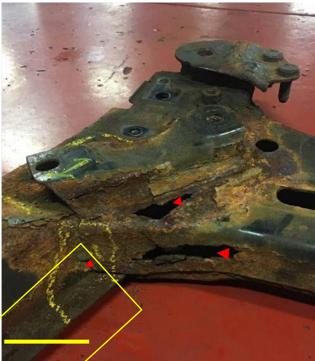
Inside Top View: Damaged Cross member
