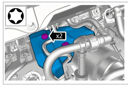
Remove the screws. Remove the marked part.
