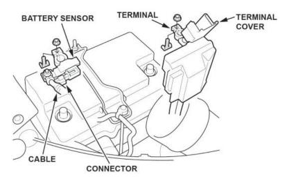
2. While holding down the terminal, torque both positive and negative clamps to 4-6 N·m (35-53 lb-in).
