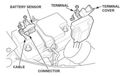
2. While holding down the terminal, torque both positive and negative clamps to 4-6 N•m (35-53 lb-in).
