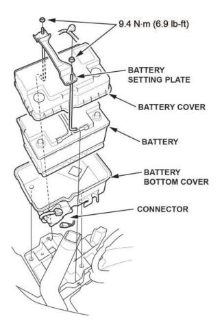
5. Install a new battery. Then reinstall the battery cover, and the setting plate in the reverse order of removal.
