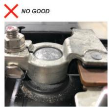
2. While holding down the terminal, torque both positive and negative clamps to 4-6 N-m (35-53 lb-in).
