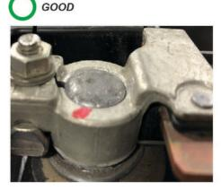
Do the battery terminals look like the good example? Yes - Go to step 2. No - Go to TERMINAL REPAIR.
