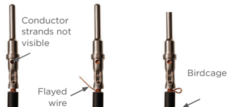
Unacceptable Crimps
