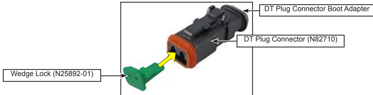
Figure 13 - Wedge Lock Insertion into Deutsch DT Plug Connector
