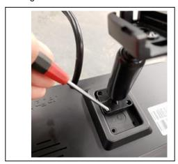
2. Install the Mirror Mount to the new Monitor using the same screws.
