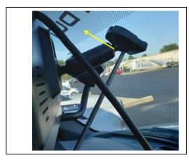
2. Once loose, slide the monitor UP to remove it from the Windshield.
