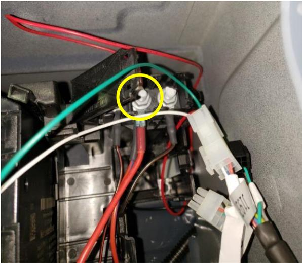
4. If the only Battery/Constant Power location available is at the Fuse Box, an Add-a-Fuse Circuit can be used (example shown below). However, it should be noted that an Add-a-Fuse Circuit is **not included**.
