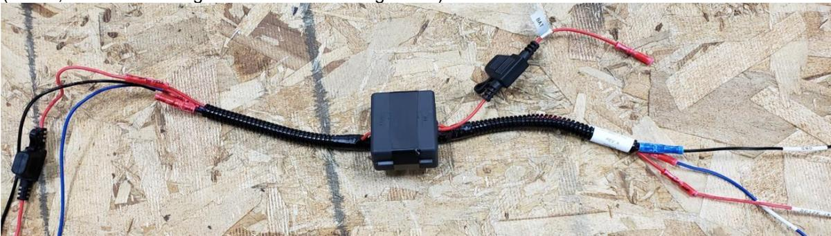
3. The Battery Wire then needs to be attached to a Battery/Constant Battery source. This could be achieved by attaching a ring terminal to a Battery Terminal at the Battery location or splicing into a Battery Wire with a Butt-connector.
