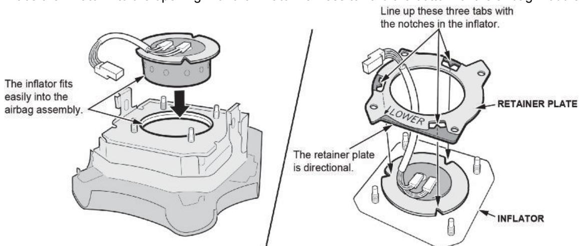
10.4.2. Install the bracket onto the studs with the stamp LOWER at the bottom of the airbag module.
