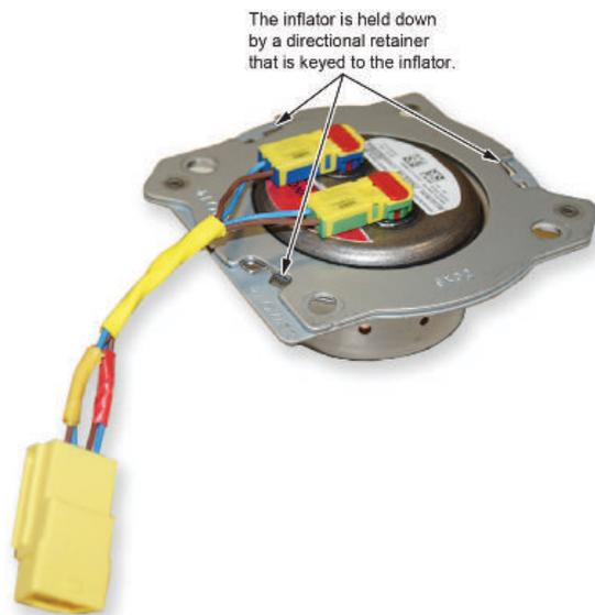
10.4.1. Place the inflator into the opening with the inflator harness toward the bottom of the airbag module.
