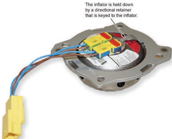
10.3.1. Place the inflator into the opening with the inflator harness toward the bottom of the airbag module.
