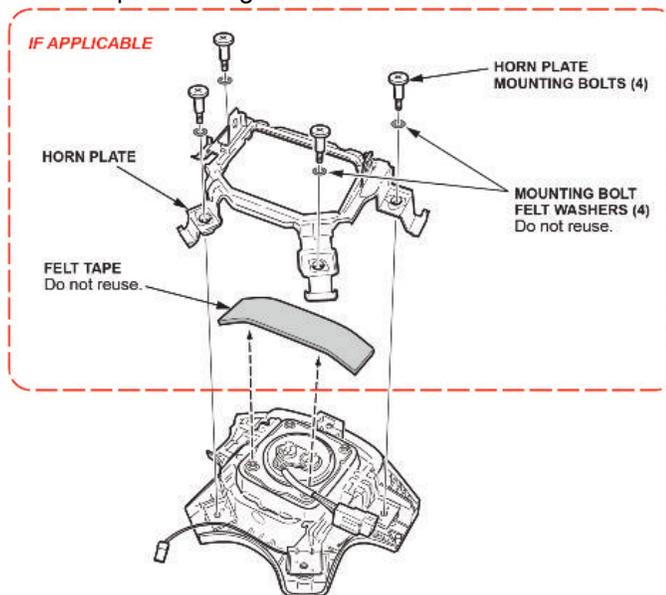
6.2. Cut the horn plate - Only for CR-V.
