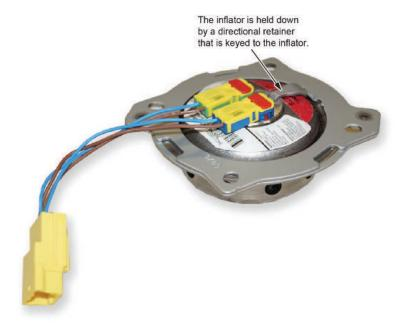
10.2.1. Place the inflator into the opening with the inflator harness toward the bottom of the airbag.
