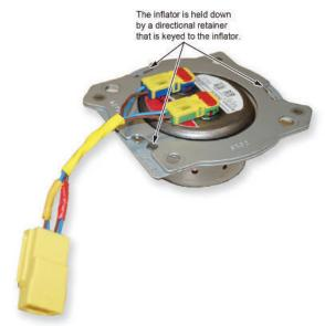
10.3.1. Place the inflator into the opening with the inflator harness toward the bottom of the airbag.
