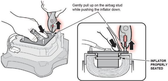
10.3. Type 4 - Check your part number against the ones listed for each installation procedure. Use the correct installation procedure for the part you received.
