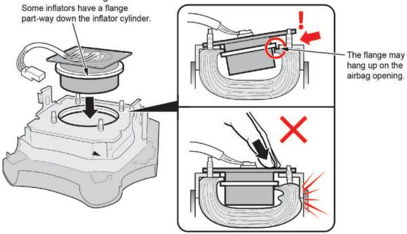
10.2.2. Using a pair of pliers, gently pull up on each stud up while pushing the inflator module down until the airbag is properly seated within the airbag module, then go to step 11.
