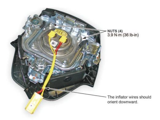
10.1.2. If the airbag inflator kit came with a label, attach the label to the inflator module as shown, then go to step 11.
