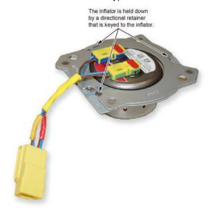
10.3.1. Place the inflator into the opening with the inflator harness toward the bottom of the airbag module.
