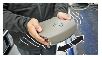
10. Install the new inflator in the airbag module.
