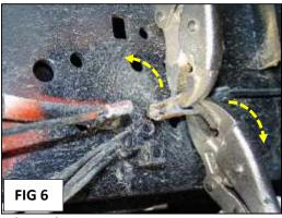
FIG 5 Clamp a second pair of vice grips next to the first pair as shown here.
