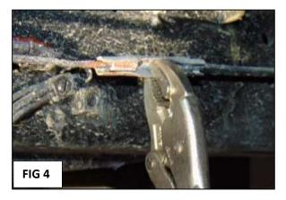
**FIG 3** Front cable clip is located rearward of the front wheels and just behind a bracket on the frame rail. **FIG 4** Clamp a pair of vice grips on the rear cable retainer as shown in this photo.
