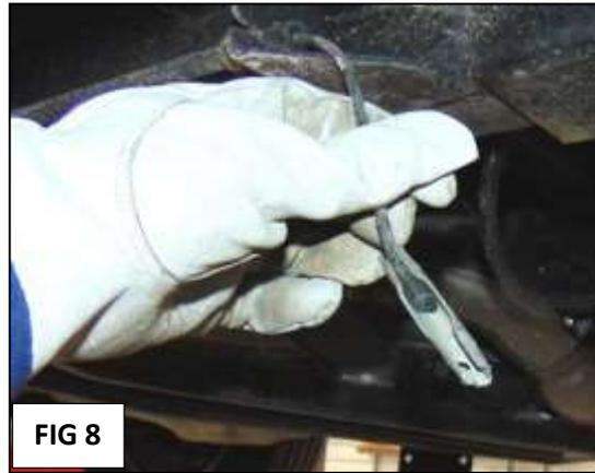
**FIG 7** Rear retainer after being spread apart showing rear cable being removed.
