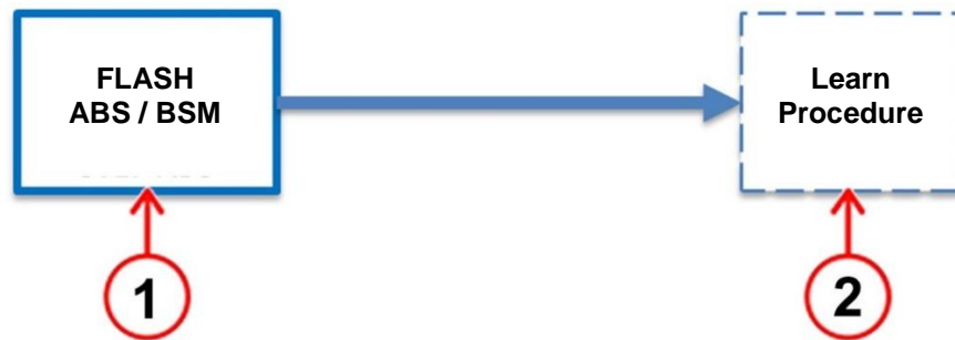
Figure 14 – ABS / BSM Software Reprogramming Sequence
