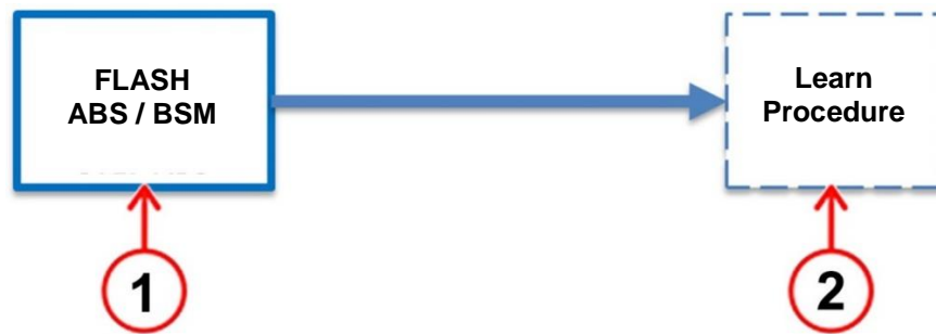
Figure 35 - ABS/BSM Software Reprogramming Sequence
