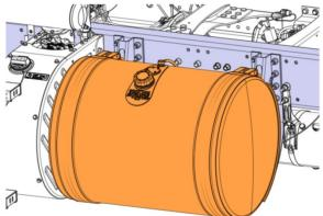
4. Locate, measure, and mark the appropriate location of the air tank brackets and mounting holes inside the frame. See the figure below for air tank location and routing.
