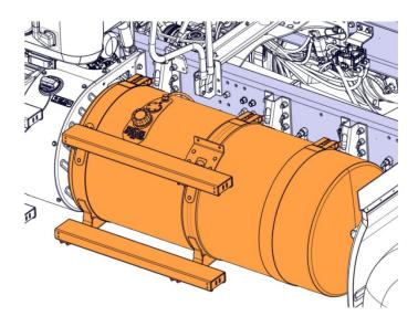
4. Remove existing 34L air tank and brackets.
