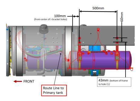
5. Drill the frame, 4 holes X 15.5 +.127 / - 0 mm (0.61 +.005 / - 0 in) Dia.
