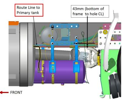
Repair Scenario 3, 18L Air Tank Alternate Location and Routing
