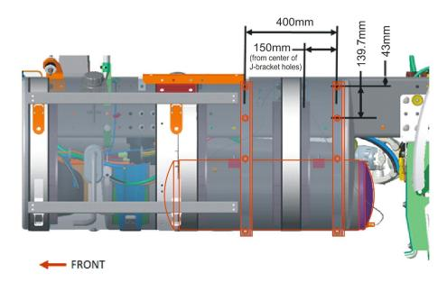
6. Drill the frame, 4 holes X 16.7 +.127 / - 0 mm (0.65 +.005 / - 0 in) Dia.
