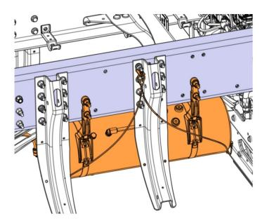
5. Locate, measure, and mark the appropriate location of the air tank brackets and mounting holes inside the frame. See the figure below for air tank routing and location.
