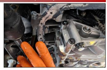
6a. Apply sealant (UM016 CH123) to the new oil pan. <u>Sealant bead width:</u> 0.08 - 0.12in. (2.5 - 3.0mm)
