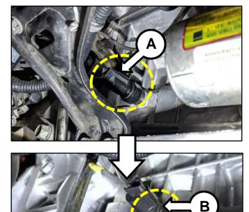
3. Install the new OPS and torque to specification and ensure the OPS connector is properly connected.
