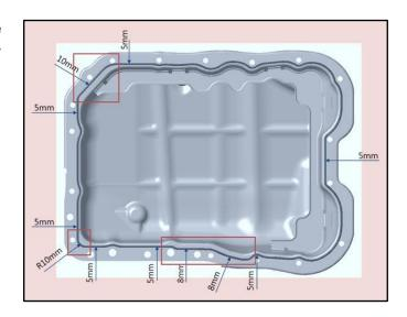
6b. Apply 2 sealant lines as wide as 0.08in (2.5mm wide) to the area where the engine block and timing cover meet as shown below. **Note**: The oil pan must be installed within five (5) minutes after application of sealant.
