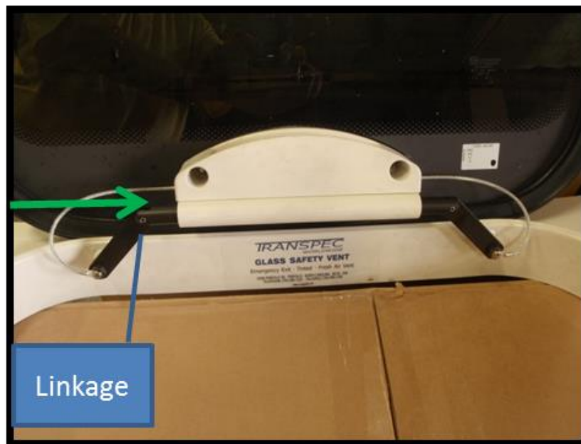
Figure 18: Re-install the left-hand linkage, ensure that the left spring is in the hinge.
