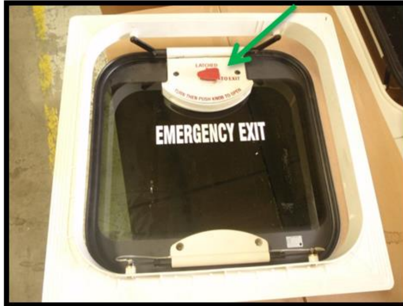
Figure 10: Rotate red release knob to the unlatched position.
