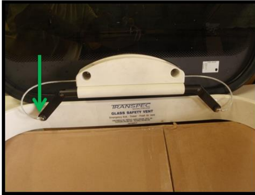
Figure 12: Remove and retain one hex bolt securing hatch linkage (green arrow, do not discard).
