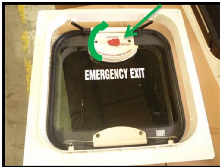
Figure 21: Rotate the red knob back to the LATCHED position.
