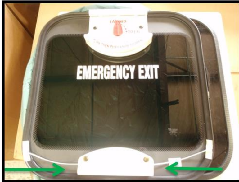
Figure 16: Install the two springs into the fixed hinge of the NEW lid, ensure all required decals have been installed.
