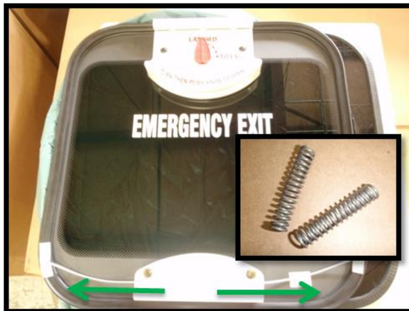
Figure 15: Retain the two springs held captive within the fixed hinge.
