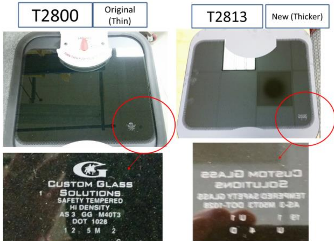
Figure 1: Original glass lid identification (left) versus new, thicker glass lid identification (right).
