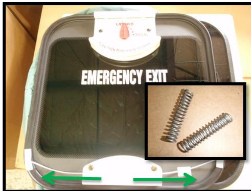
Figure 13: Retain the two springs held captive within the fixed hinge.
