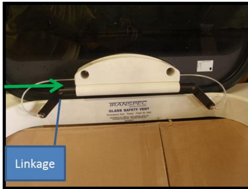
Figure 16: Re-install the left-hand linkage, ensure that the left spring is in the hinge.
