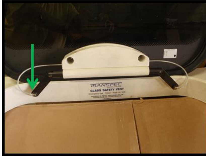
Figure 10: Remove and retain one hex bolt securing hatch linkage (green arrow, do not discard).
