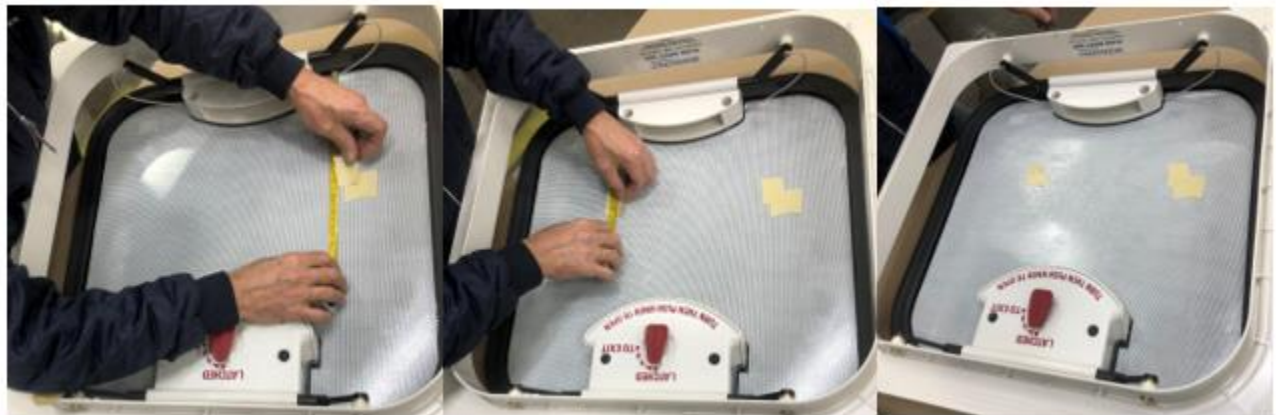
Figure 5: Mark decal location on the tint film using masking tape.
