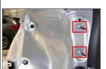
6. With the rear lights removed from the vehicle, the tail light mounting studs and vehicle body **MUST** be cleaned to remove potential residual manufacturing oil
