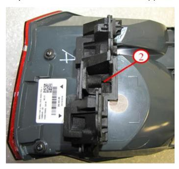
18. Install the 3 self-tapping screws into the inner and outer holders, following the tightening order shown below of 1-2-3. Ensure that both holders are held tightly against the tail light during installation of the screws.
