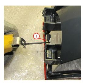
5. De-burr all of the plastic edges from cutting during the previous steps. Using compressed air, ensure that all of the plastic debris is removed. The tail light must be completely free of any cutting remains.
