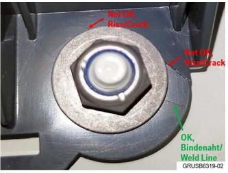
Ensure the tail lights are only replaced in case of cracking.
