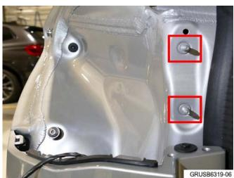
6. With the rear lights removed from the vehicle, the tail light mounting studs and vehicle body MUST be cleaned to remove potential residual manufacturing oil.
