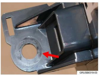
5. With the tail lights removed, re-inspect both sides of the tail light mounting tabs for signs of cracking.
