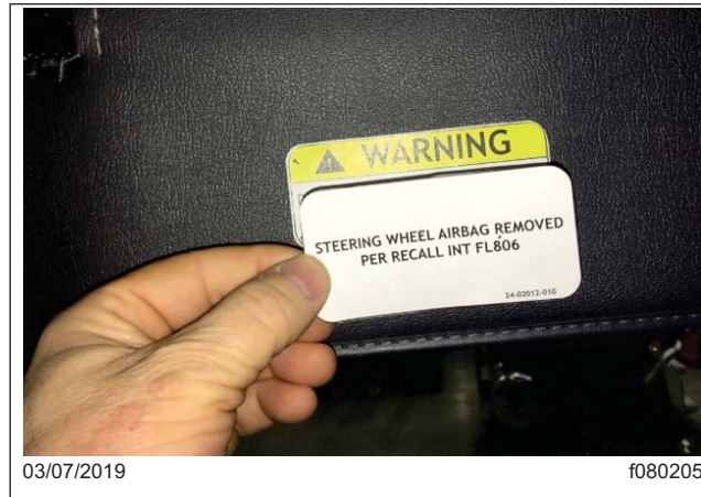
Fig. 15, Installing the Stickers on the Sun Visor
