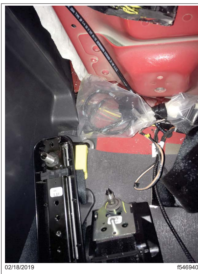
Fig. 12, Harness Secured Behind the Seat
