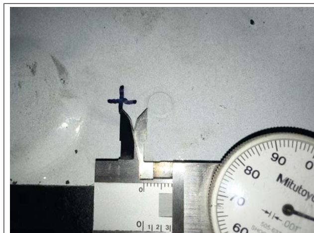
Fig. 4, Measuring Between the Floor Mound and the Rivet
