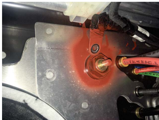
Fig. 7, GNDE Engine-Side Pass-Through Stud
