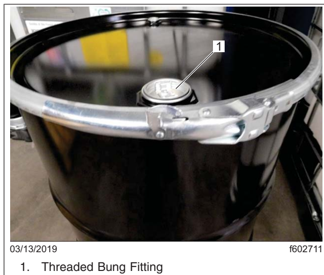
Fig. 10, Steel Drum with Bolted Ring Assembly
