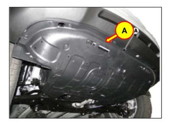
2. Inspect for engine oil leakage from the engine oil pan.
