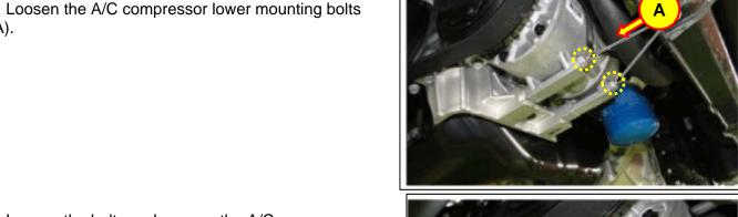
3. Loosen the bolts and remove the A/C compressor bracket (B).
