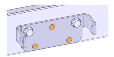
6. Remove the bracket and keep mounting bolts for assembly.
