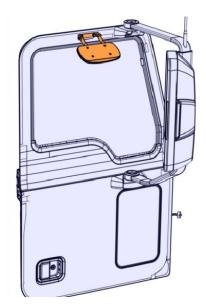
2. Remove the screws and mirror. Scrap the gasket. Retain screws for re-assembly.
