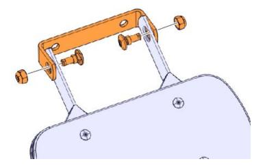
4. Install the new bracket (78537771) to be used as a template.
