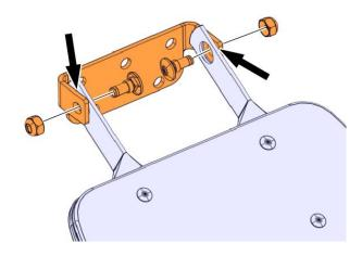
11. Install the new mirror assembly with the new gasket (78537810) using the original two bolts and three new bolts (25185871). Use hand tools to install bolts. Torque the bolts to 8 nm +/- 1.2 nm.
