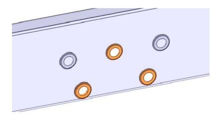
7. Install the new mirror assembly with the new gasket (78537810) and five bolts (25185871). Use hand tools to install bolts. Torque the bolts to 8 nm +/- 1.2 nm.
