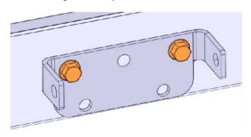
3. Drill the three new 8 mm holes in the door using the bracket as a guide
