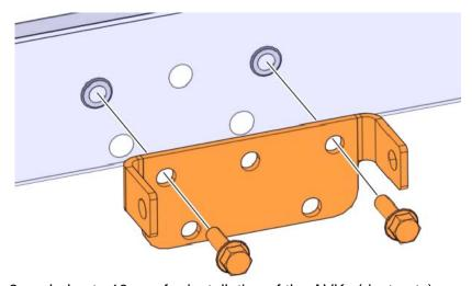
5. Enlarge the 8mm holes to 10 mm for installation of the AVKs (rivet nuts).
