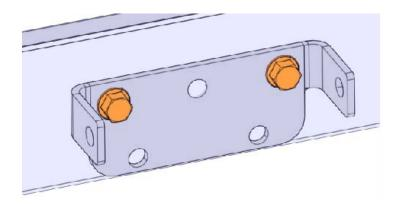
Drill the three new 8 mm holes in the door using the bracket as a guideNote: Use a drill stop set to only penetrate the outer sheet metal.
