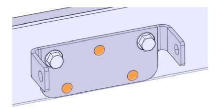
4. Remove the mirror and bracket and keep mounting bolts for assembly.
