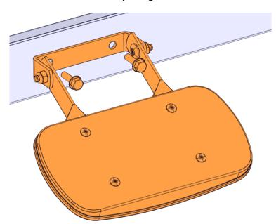
3. Remove the screws and original bracket. Scrap the bracket. Retain the nylon washers and screws.
