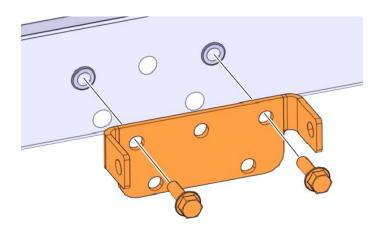
7. Enlarge the 8mm holes to 10 mm for installation of the AVK (rivet nuts).
