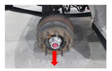
**5**. Push down on the lower brake shoe. Pull on the cam roller retainer clip to disengage the retainer and cam roller from the brake shoe. Remove the lower brake shoe cam roller. Discard the cam roller.
