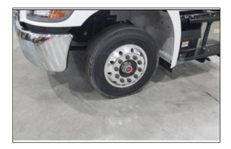
**24**. Tighten the front wheel lug nuts on both sides of the vehicle to the specified torque.
