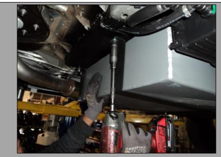
20. Torque the four fuel tank strap bolts to 30 ft-lbs then mark the bolts with a paint stick to indicate they have been torqued
