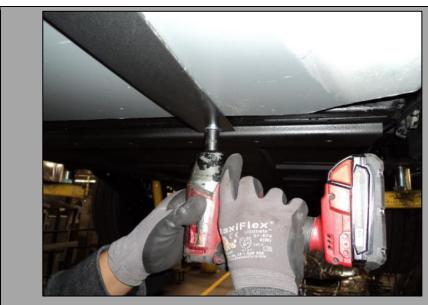
18. At the front of the tank, align the passenger side tank strap with the beveled edge of the tank as shown
