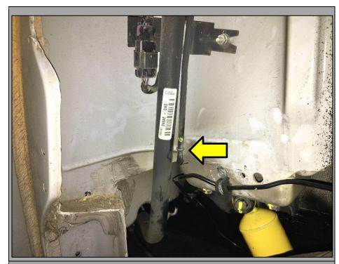
8. At the driver side rear corner of the tank, use a 10mm socket to loosen the hose clamp around the filler neck. Remove the rubber hose from the fuel tank.
