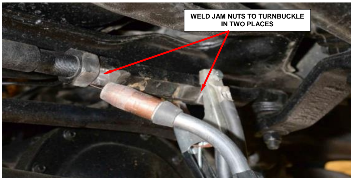
Figure 9 – Weld Both Jam Nuts to the Turnbuckle
