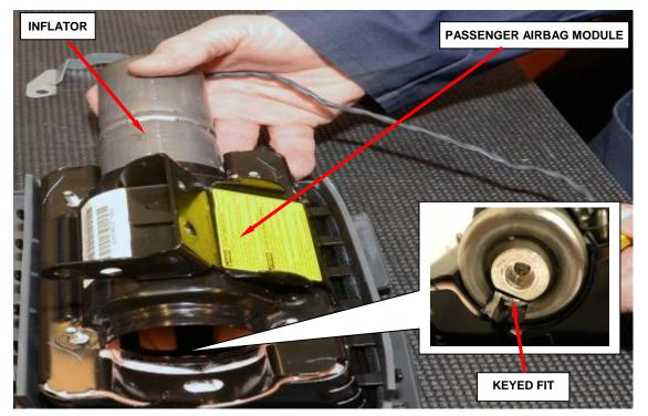
Figure 22 – Passenger Airbag Inflator to Housing
