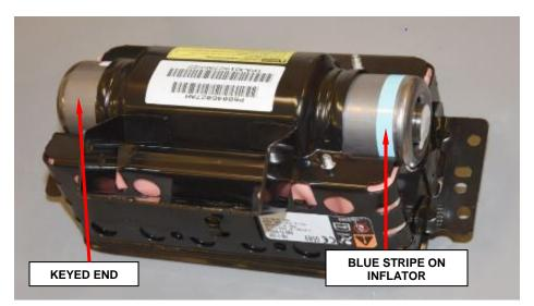
Figure 34 – Insert Inflator (Shown with Cushion Installed)
