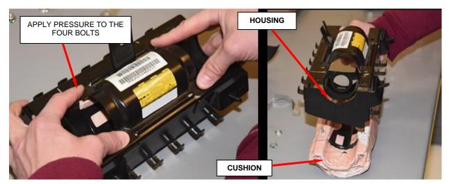
Figure 105 – Remove Airbag Cushion from Housing
