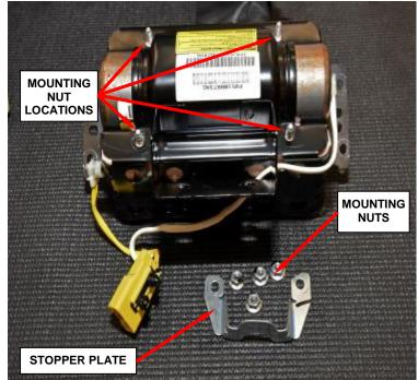
Figure 51 – Mounting Nuts and Stopper Plate
