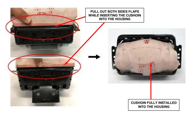
Figure 57 – Side Flaps Must Be Held Out
