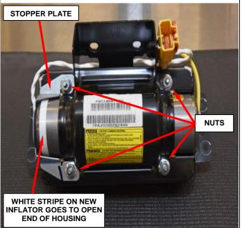
nuts to the airbag housing and tighten to 53 in. lbs. (6 N⋅m) (Figure 60).
