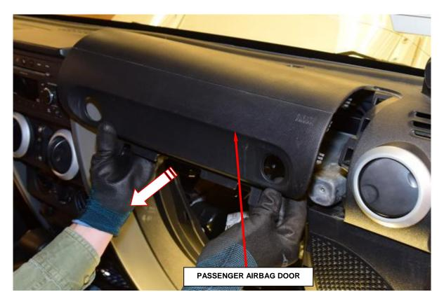
Figure 92 – Passenger Airbag Door
