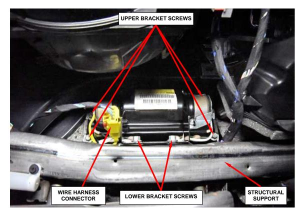
Figure 45 – PAB Housing, Inflator and Cushion to be Removed a Unit (View through Glove Box Opening)
