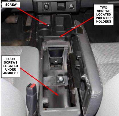
Figure 63 – Floor Console (ATX Shown)
