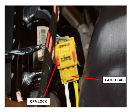
Figure 82 - Airbag Inflator Pigtail Connector
