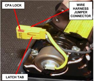
Figure 14 – Wire Harness Jumper
