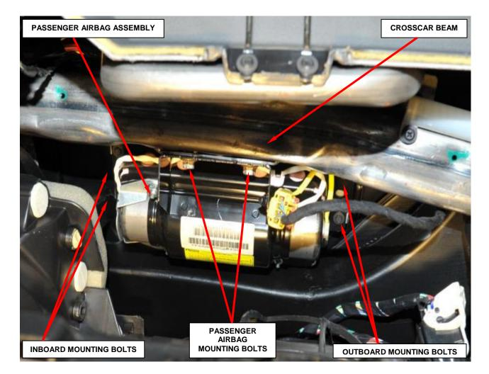
Figure 13 – Passenger Airbag Mounting Locations
