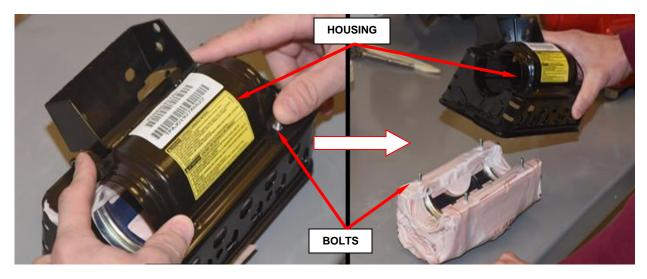
Figure 31 - Remove Airbag Cushion from Housing
