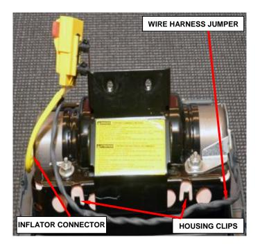
Figure 15 – Wire Harness Jumper
