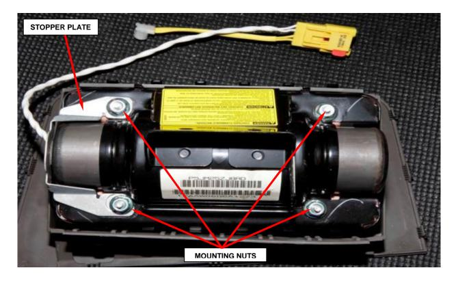
Figure 86 – Mounting Nuts and Stopper Plate
