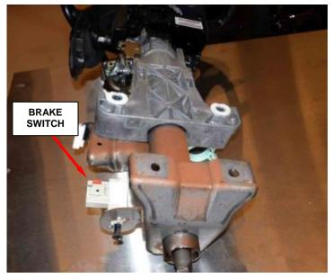
Figure 67 - Brake Switch Connector (Column out of Vehicle for Photographic Purposes)
