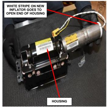
Figure 58 – Install New Inflator to Housing
