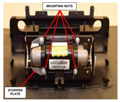
Figure 103 – Mounting Nuts
