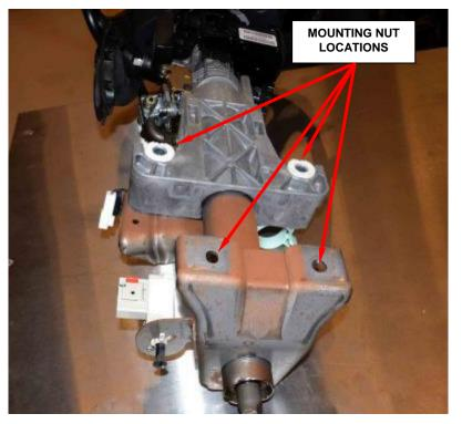
Figure 71 - Steering Column Mounting (Column Removed for Photographic Purposes)
