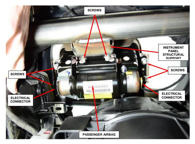
Figure 28 – Passenger Airbag
