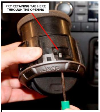
Figure 95 - HVAC Outlet Tab
