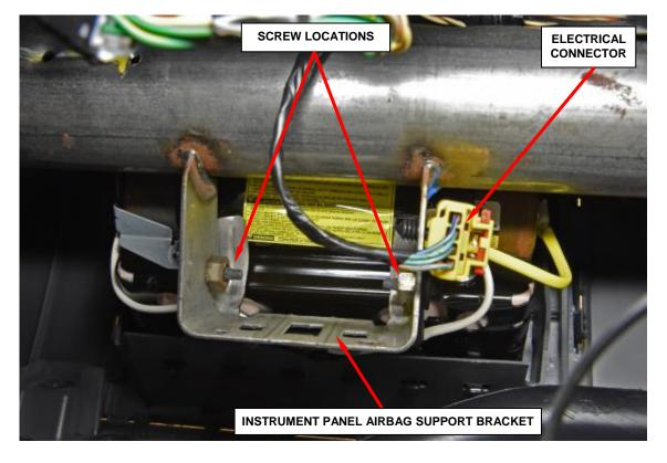
Figure 3 – Airbag Module (View through glove box opening)
