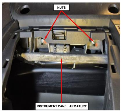
Figure 91 – Lower Passenger Airbag Nuts
