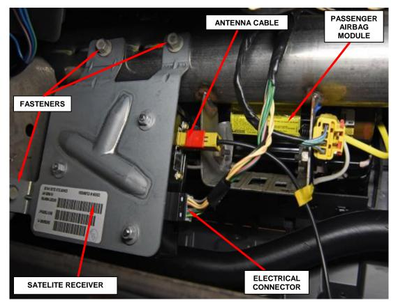
Figure 2 – Satelite Receiver (if equipped) (View through glove box opening)
