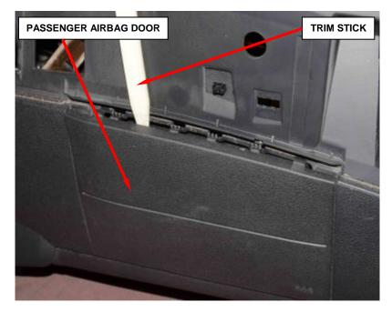
Figure 83 – Passenger Airbag Door
