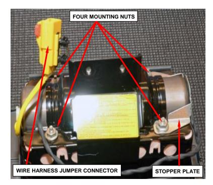
Figure 16 – Airbag Module
