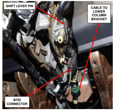
Figure 69 – Gear Shift Cable
