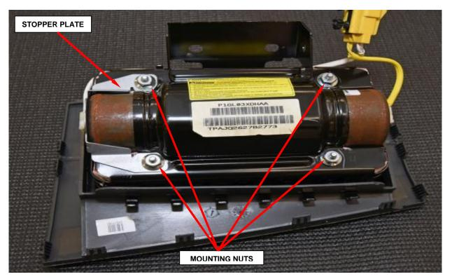
Figure 7 – Mounting Nuts and Stopper Plate
