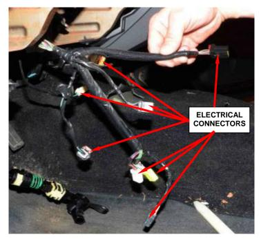
Figure 68 – Column Electrical Connectors
