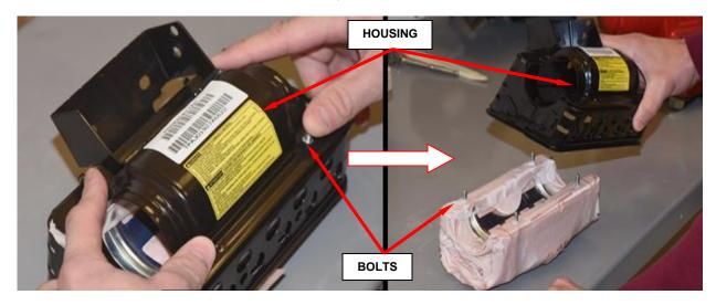
Figure 53 - Remove Airbag Cushion from Housing
