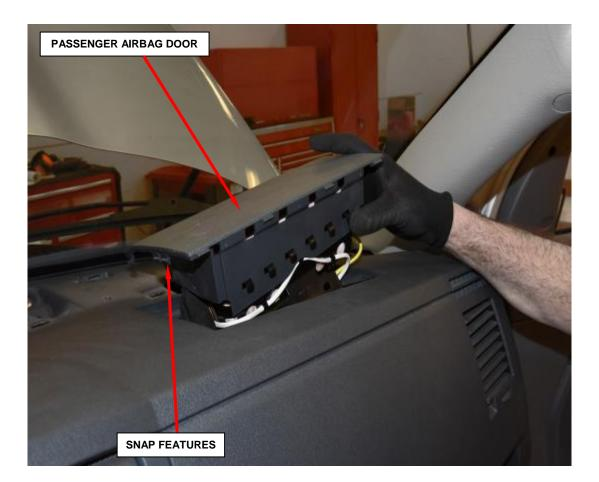
Figure 4 – Passenger Airbag Removal
