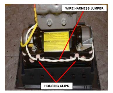
Figure 84 – Passenger Airbag Assembly
