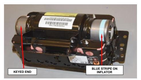
Figure 20 – Insert Inflator (Shown with Cushion Installed)
