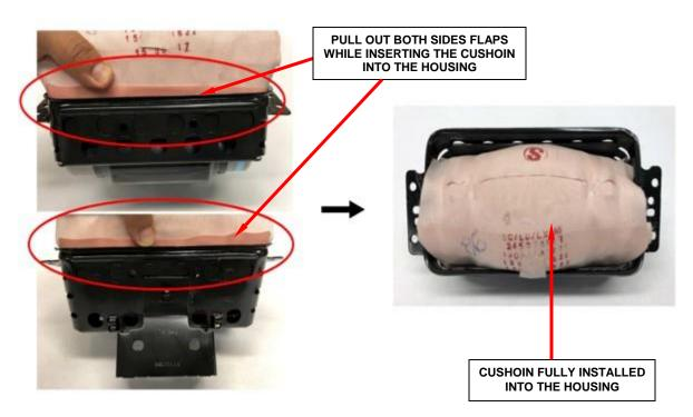
Figure 21 – Side Flaps Must Be Held Out
