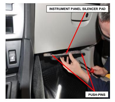
Figure 10 - Instrument Panel Silencer
