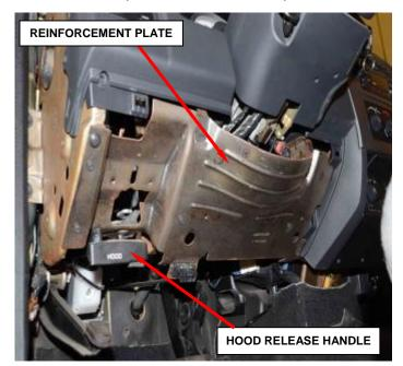
Figure 65 – Steering Column Reinforcement Plate
