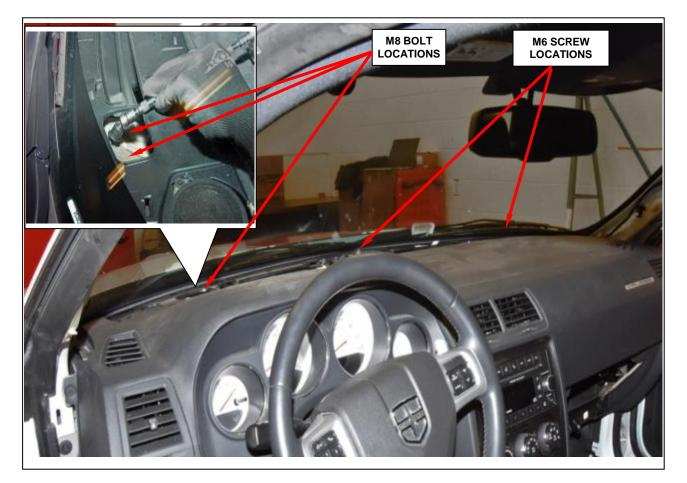
Figure 46 – Top Instrument Panel Fasteners
