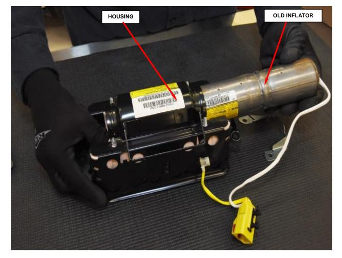
Figure 52 – Passenger Airbag Inflator Removal
