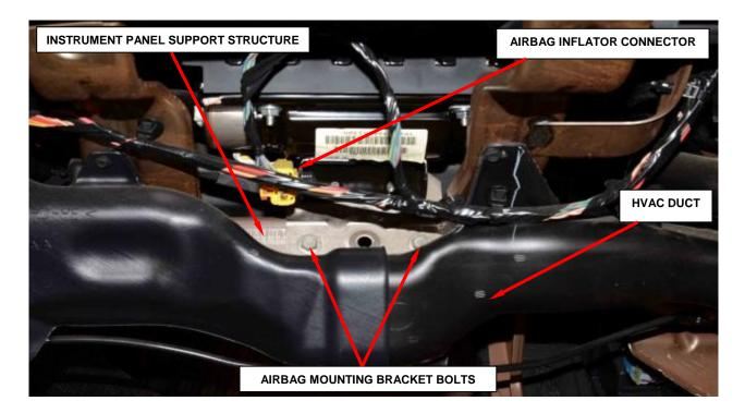
Figure 81 – Instrument Panel Mounting Bracket
