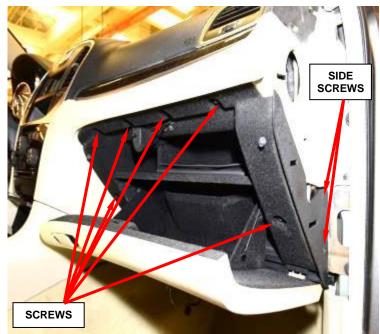
Figure 25 – Glove Box Compartment
