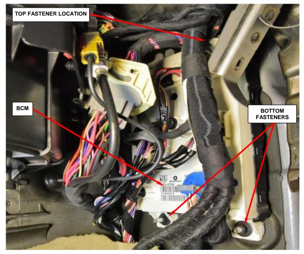
Figure 26 – Body Control Module
