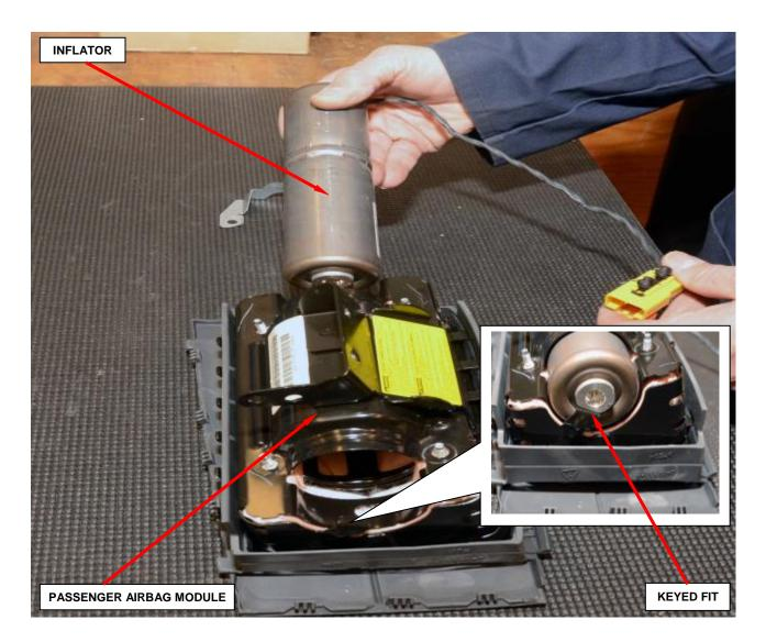
Figure 88 – Passenger Inflator Installation
