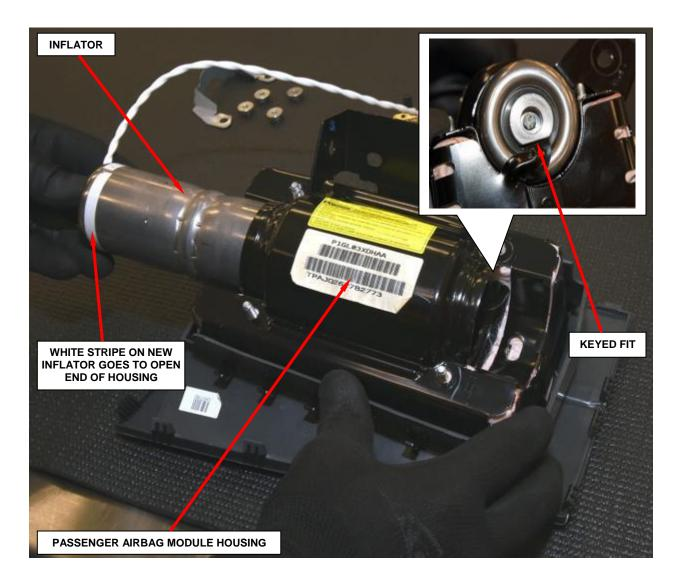
Figure 9 – Passenger Inflator Installation
