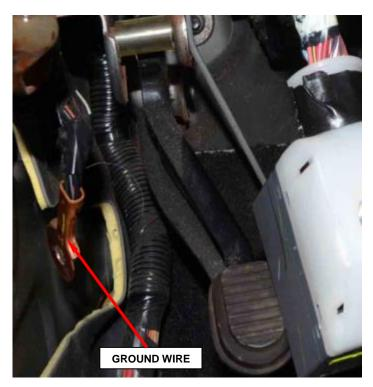
Figure 74 – Bolt and Ground Location
