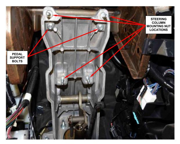
Figure 72 – Pedal Support Bolts
