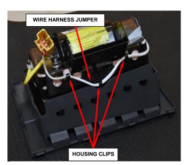
Figure 6 – Wire Harness Jumper
