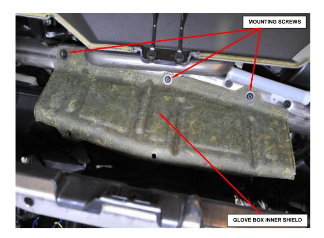
Figure 12 – Inner Glove Box Shield
