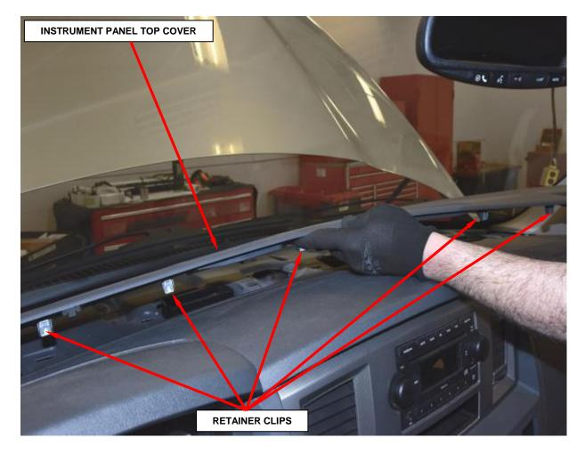
Figure 1 - Instrument Panel Top Cover
