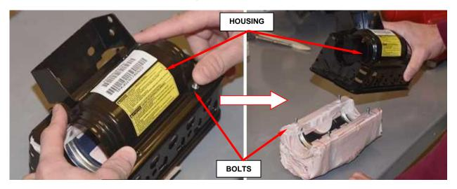
Figure 17 - Remove Airbag Cushion from Housing
