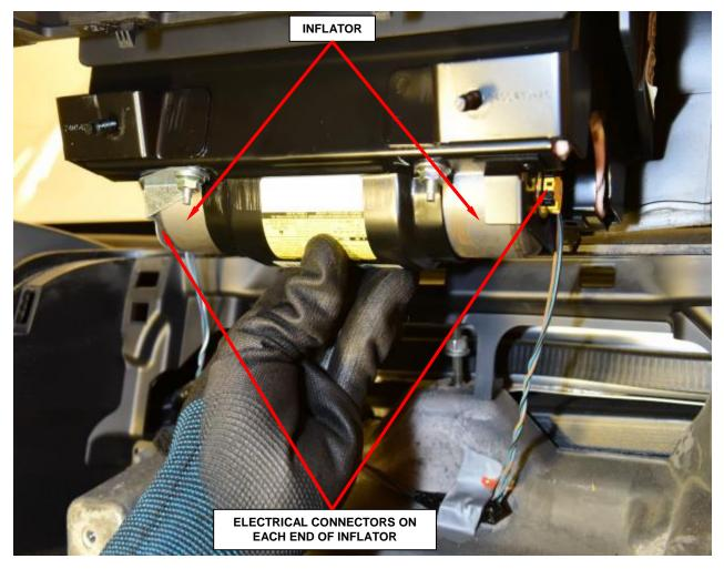
Figure 93 – Airbag Inflator Electrical Connectors
