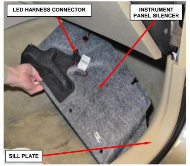
Figure 24 – Instrument Panel Silencer
