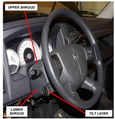
Figure 66 – Steering Column Shrouds
