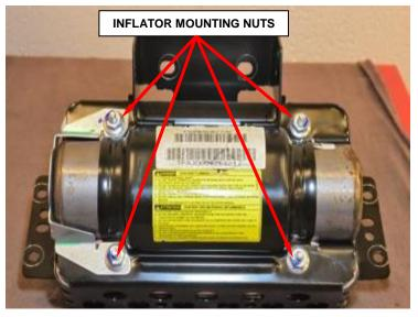
Figure 29 – Mounting Nuts
