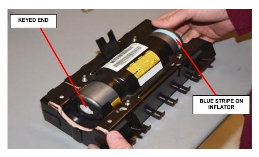
Figure 108 – Insert Inflator (Shown with Cushion Installed)
