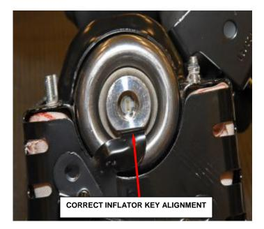
Figure 61 – Check for Inflator Key Alignment
