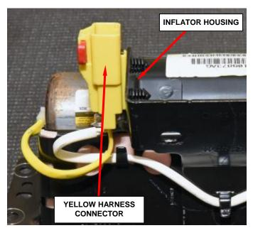
Figure 49 – Wire Harness Connector
