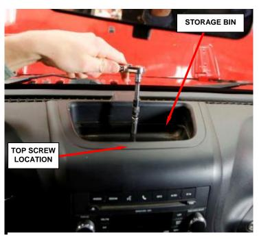
Figure 97 – Center Bezel Screws
