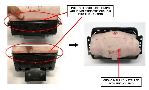
Figure 35 – Side Flaps Must Be Held Out
