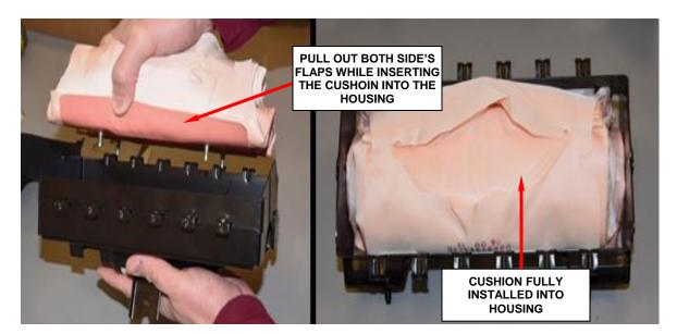
Figure 109 - Side Flaps Must Be Held Out
