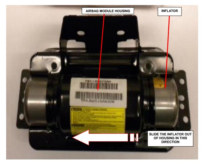
Figure 36 – Remove Airbag Inflator
