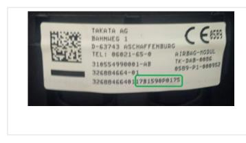
It is necessary to document which air bag goes into which vehicle. Therefore the technician is required to note on the repair order the serial number of the new air bag.
