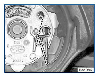
Insert Torx screwdriver (T20) roughly straight from below into opening on reverse side of steering wheel up to stop (approx. 5.5 cm). Swing Torx screwdriver (T20) with handle sideways until airbag unit is unlocked.
