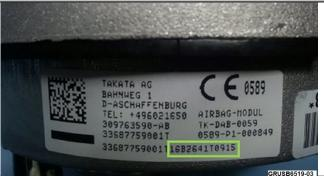
Before installing the replacement part, the new air bag module's serial number (circled) must be documented by the technician on the repair order so it can also be entered into the warranty claim's comment section.
