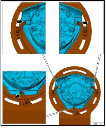
Clamp airbag centrally in airbag support. There are securing points on the sides <arrows>, parallel, opposite each other, and below.
