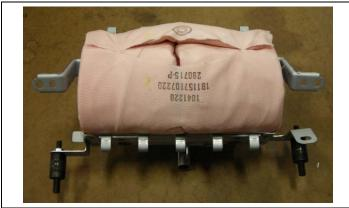
a) Mount the adaptors (579943-3R3) to the airbag as shown.
