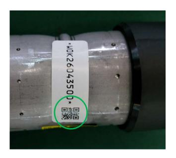
c) If the inflator serial number cannot be scanned or is not present check the box as shown below.
