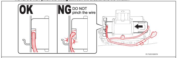
NOTE: Ensure the inflator is correctly oriented.
