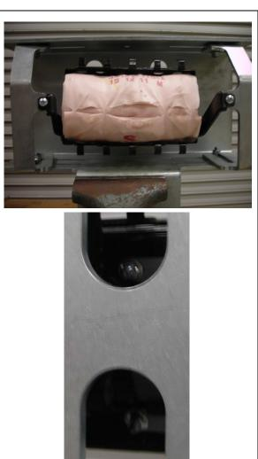
f) Mount the airbag into the mounting bracket as shown.
