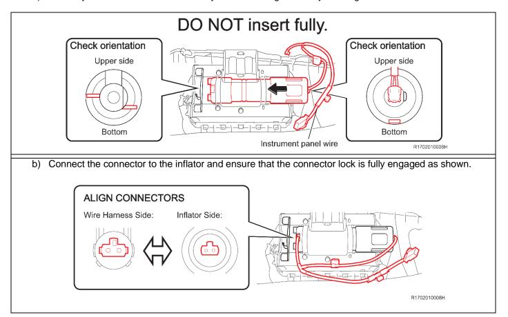
a) Fully insert the inflator and ensure that the inflator is correctly orented as shown. NOTE: DO NOT pinch the wiring between the bracket and the inflator.
